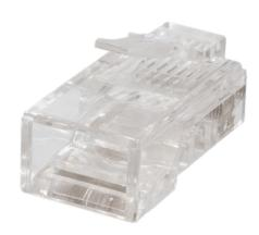
Category 5e Contractor Grade 5925 RJ45 Plug (PXSPDY5b): plugs are designed to simplify twisted pair terminations by allowing the wire pairs to be easily inserted through the plug and out of the front. This allows the installer to easily check the wiring order before crimping the connector. Twist is maintained more easily enabling a better performing crimp. Waste is minimised and the plugs are suitable for either stranded or solid wires.
